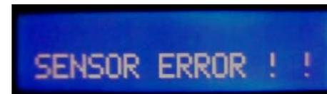
The message blinks continuously indicating sensor malfunction. In this situation, the boiler heaters are turned off immediately and any unit manipulation is not possible. This requires thermostat servicing.
