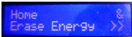
The operator is expected to make a selection. If at this point the
