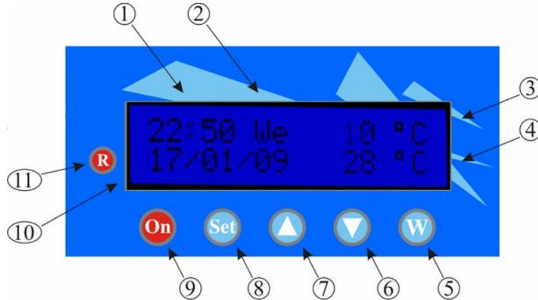
The thermostat K043-D was manufactured with a purpose of boiler management and reduction of electrical energy consumption. It contains ten built-in memories and one weekend memory. The different memory settings regulate the working conditions of the boiler heaters. They can be pre-set according to the settings of the local electrical energy supplier and the legal tariff system. The thermostat has relay to operate boiler heater of 1,5 kW and achieve economy mode operation.
