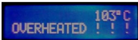
The message blinks continuously indicating there is an error in the system, showing at the same time the water temperature. In this situation, the boiler heaters are turned off immediately and any unit manipulation is not possible. If water temperature drops below 92°C, the unit returns to the main menu and
