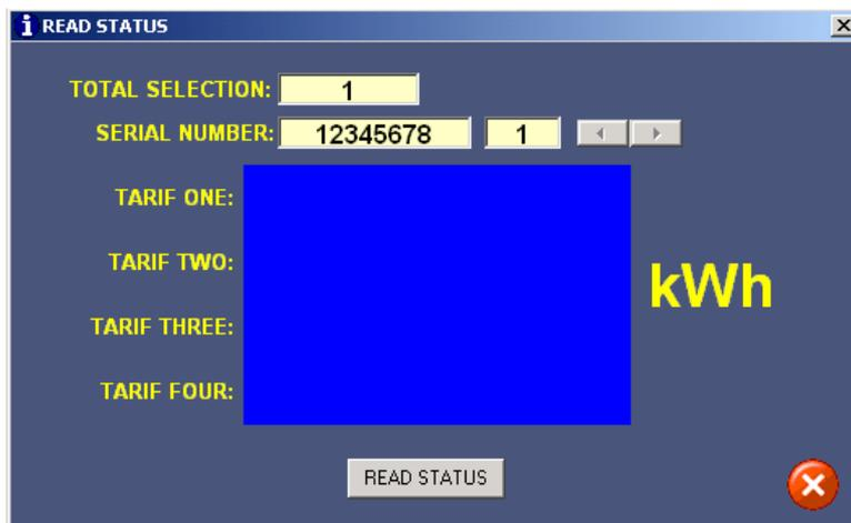
The STATUS command enables registration of the total energy consumed by the customer. To read the status simply press the 'READ STATUS' button. The records are automatically saved in the database. The database holds the last 15 records, for each of the four tariffs. By clicking the serial number on the Tree View or List View, these records are automatically shown in the Customer Details Area.
